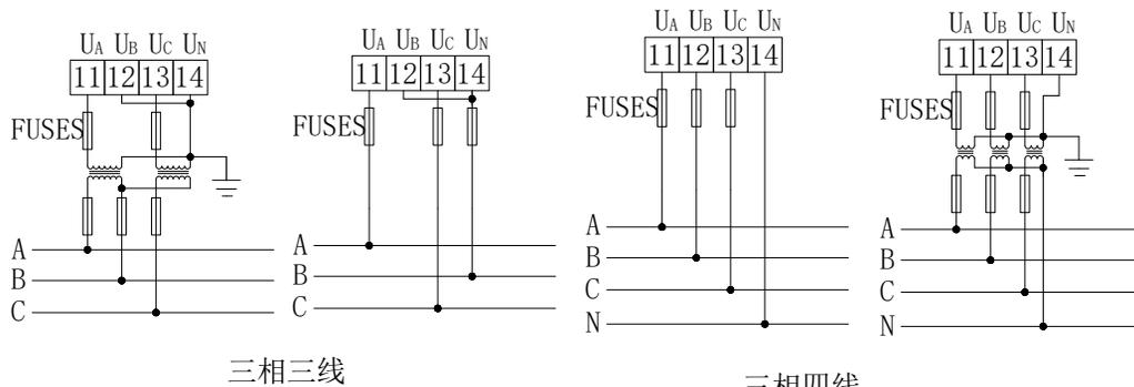
AMC72/96电压接线
